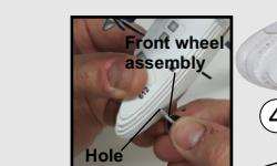
Insert the front wheel assembly into the hole at the front of the fuselage.
