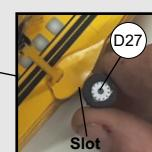
Insert rear landing gear into the slot in the fuselage.
