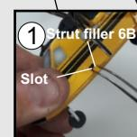
Slide the front strut filler part 6B into the front slot.
